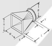
**Hood Design Basis:** 150 fpm capture velocity 2 ft. distance from source
